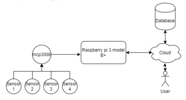
The data from the water level sensor will allow the microcontroller to automatically turn on the pump when the water level is below a certain level and turn off the pump when the water level is above a certain level.
